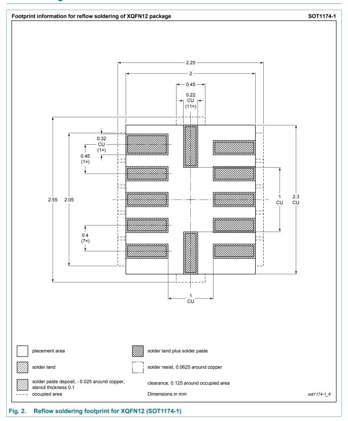
plastic, leadless extremely thin quad flat package; 12 terminals; 0.4 mm pitch; 1.7 mm x 2 mm x 0.5 mm
