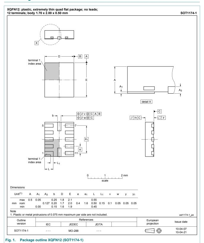
plastic, leadless extremely thin quad flat package; 12 terminals; 0.4 mm pitch; 1.7 mm x 2 mm x 0.5 mm body
